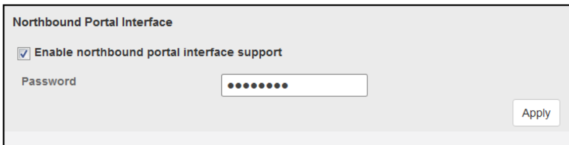
FIGURE 11 Enabling Northbound Portal Interface Support on ZoneDirector
